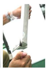
The troffer frame is mainly composed by ABS material mixed with other fireproof material, which can prevent or block the flame from spreading. The test proves that the fireproof performance is superior, completely unable to burn.
