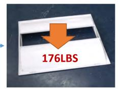
Troffer adopt high-performance synthetic material, it can bear about 176 lbs without any transformation. Though the frame deform because of unilateral compression, it resumes once released, no signs of aging at all.
